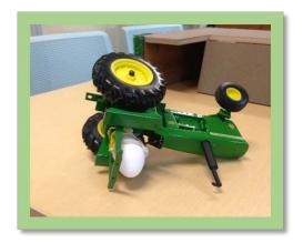
The results of the second tractor with a ROPS demonstrates that when the tractor tips the egg remains in the tractor and is protected by both the ROPS and by wearing a seatbelt. This demonstration provides a great visualization for kids to see the difference a ROPS can make in preventing injury to the tractor operator and teaches them about the center of gravity of large farm machinery.
